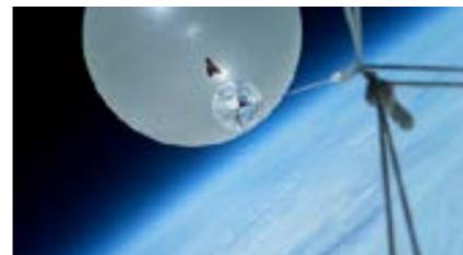
The Earth viewed at an altitude of nearly 30 kilometres. The 7 meter diameter weather balloon, parachute and radar reflector are visible. This photo was taken with the upward facing camera.
